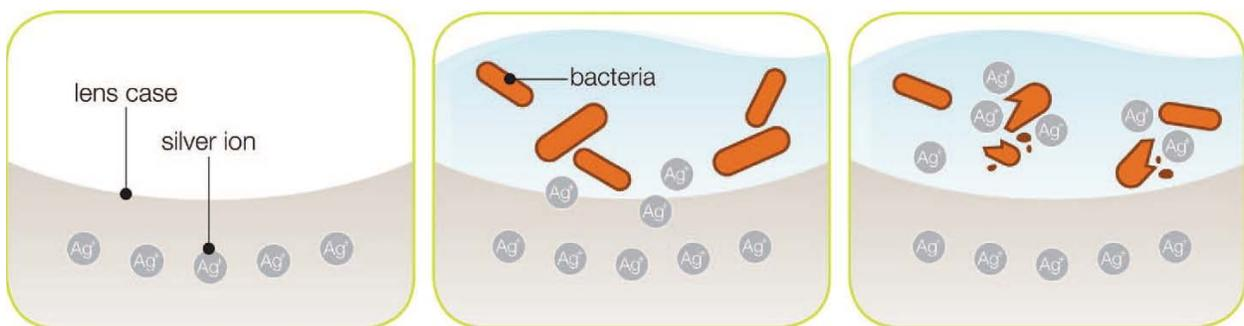
Fig 3: Silver impregnated lens case works by slowly releasing silver ions into the solution to maintain an antibacterial surface.
